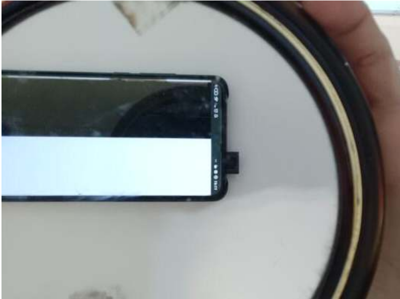
Figure 4.13: Image capturing with a mirror to reflect the screens state at the time of imaging
