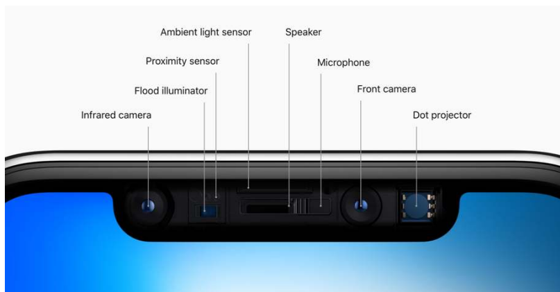
Figure 1.2: There are a multitude of sensors on the iPhone, providing high accuracy. 2
